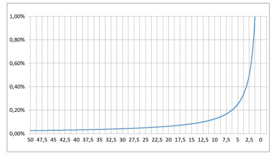
Usage of 5 N load cell = 0.25 N–5 N with accuracy of +/- 1 %, resolution of individual measured value = 0.00125 N
