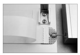
3. Place the end of the test strip centrally on the sample clamp and fix it with the clamping lever. When released, the clamping lever folds back into the starting position.
