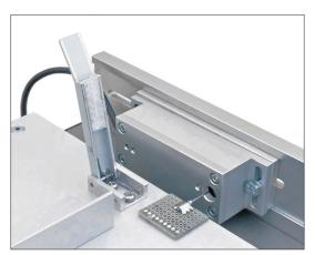
The force acting on the load cell is converted into an electrical signal and amplified.
